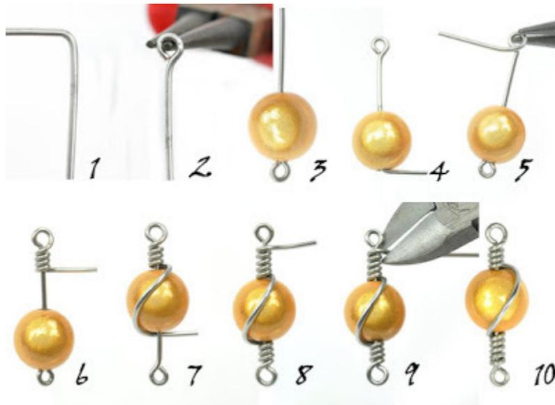
Step 1 Cut 20cm length jewelry wire. Bend one side of the wire and form a right-angle.
